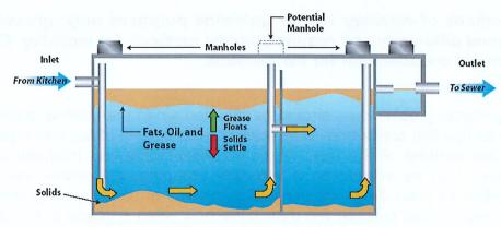
CONVENTIONAL GREASE INTERCEPTOR Outdoor, In-ground-Precast Concrete (Typical)
