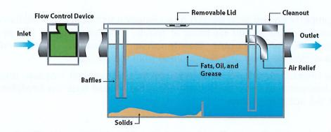
**GREASE TRAP** Indoor, Above Ground (Typical)
