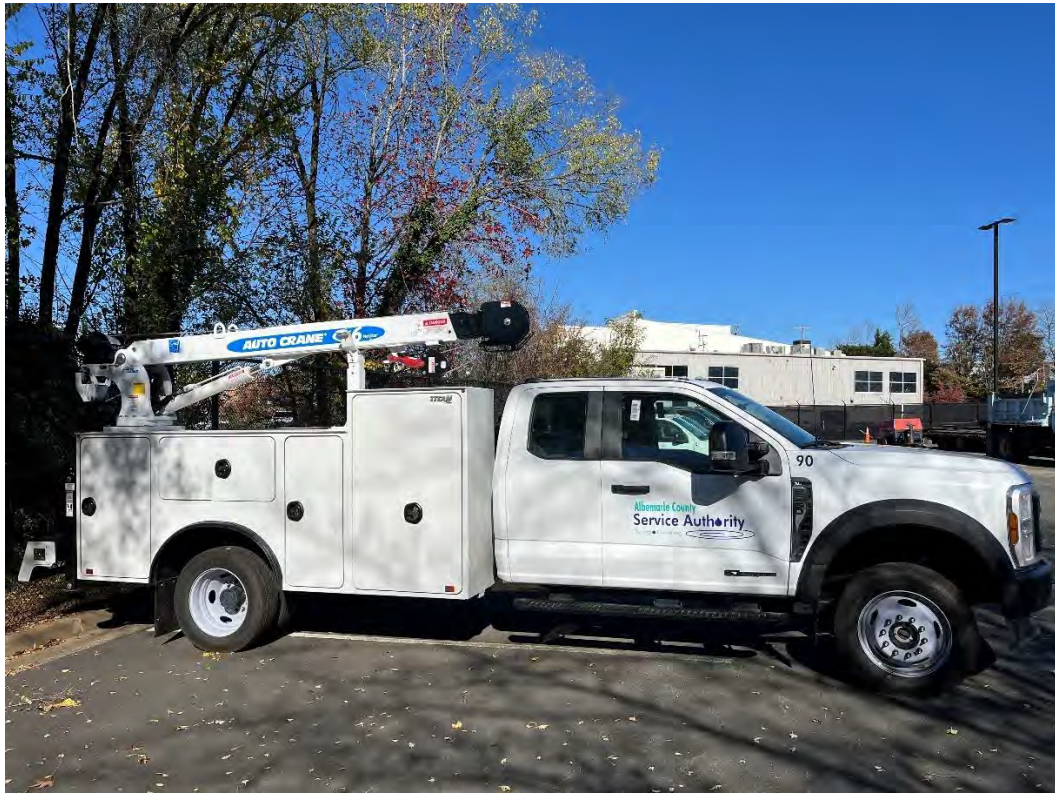
Attachment 4: Unit 90 – Ford F-550 Utility Truck with 3-Ton Crane
